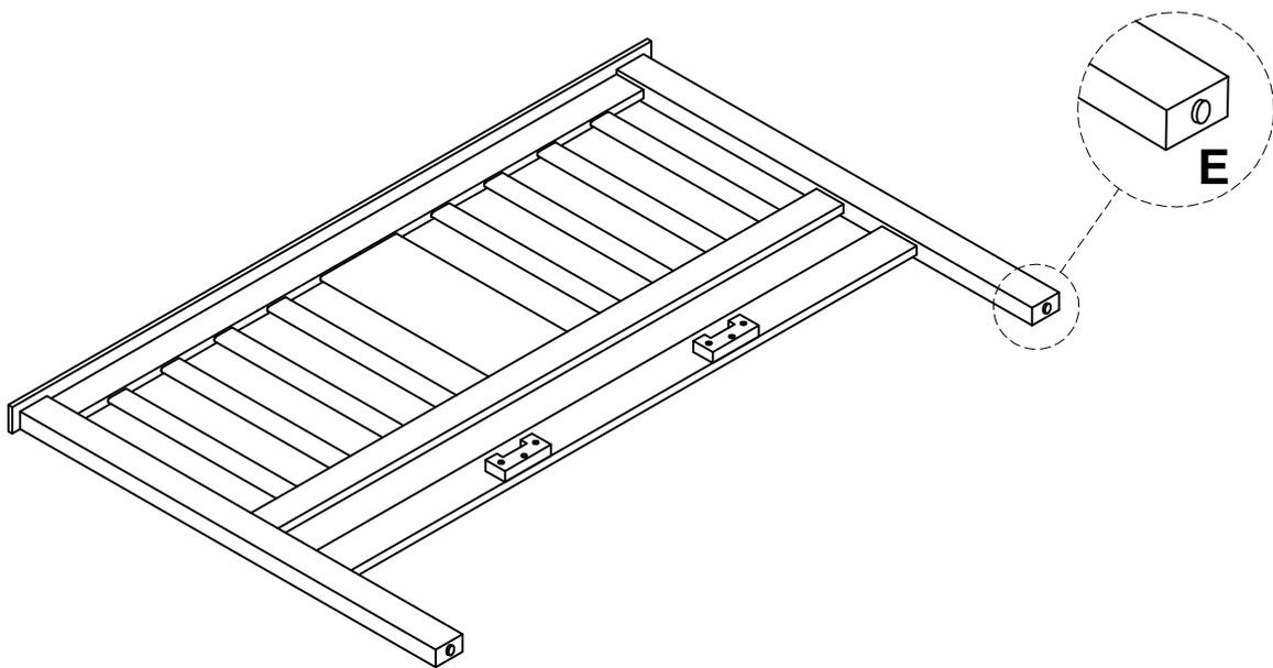
STEP 1: Attach 3 onto 1 and 2 using the bolts (B), tighten it up by using an allen key (D)
