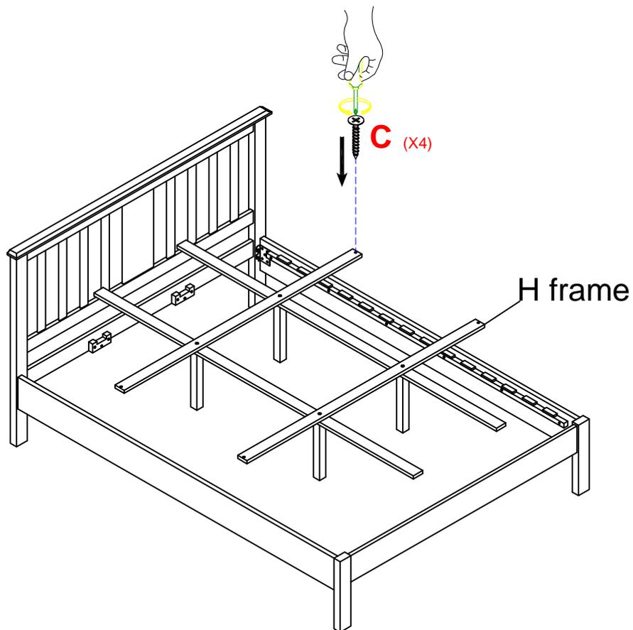
STEP 4: Attach **7** onto **3** using the screws (**C**), tighten it up by using a screwdriver.
